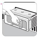
Clean it with a brush and rinse it under the shower if necessary. Also clean the outside, removing all fluff. Clean the rubber seal round the condenser cabinet and in the inner part of the small door with a damp cloth.
